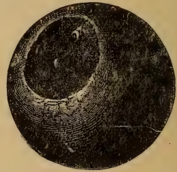
FIG. 160.—SPHERULE WITH METALLIC NUCLEUS COATED WITH BLACK MAGNETITE, SUPPOSED TO BE OF COSMIC ORIGIN ("CHALLENGER").
